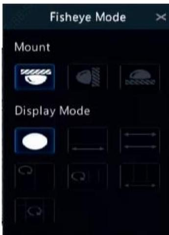
Three mounting modes are available: ceiling, wall, desktop. Ceiling and desktop mounting modes use the same dewarping method.
