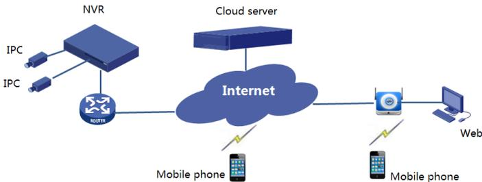
The NVR and the connected IP cameras are located on a private network (or LAN), and you manage these devices through the cloud server, a cloud solution for device management over Internet. After registering a cloud account and properly configuring your network devices (including router), you can manage your NVR and the connected IP cameras from a PC or a mobile phone.
