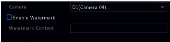
The screenshot displays a configuration panel for video watermarking. At the top, there is a 'Camera' dropdown menu with 'D1(Camera 04)' selected. Below this is a checkbox labeled 'Enable Watermark', which is currently unchecked. At the bottom, there is a text input field labeled 'Watermark Content' that is currently empty.
